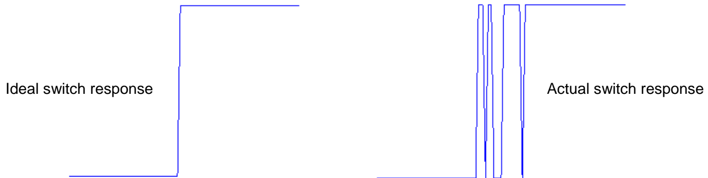
Demonstrating switch bounce
